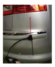
2. ALWAYS MOUNT THE ANTENNA VERTICALLY WITH THE RED COLOURED RADIAL POINTING UPWARD.
